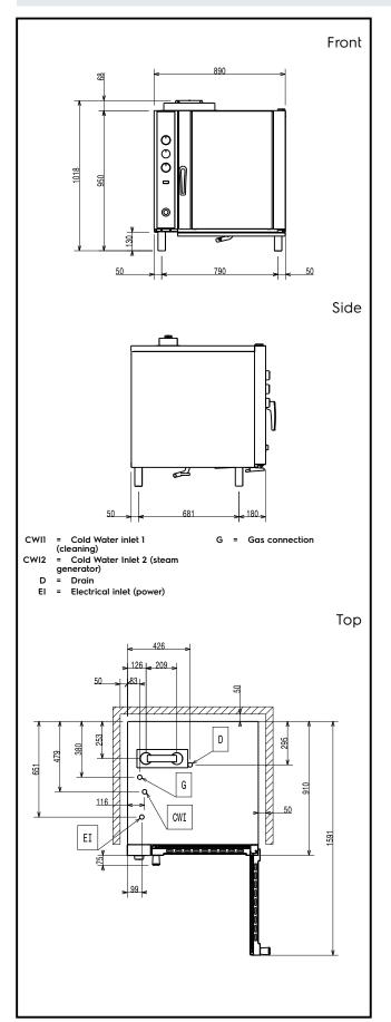
Electric Supply voltage: 220-230 V/1 ph/50 Hz Auxiliary: 0.35 kW Electrical power, max: 0.35 kW Gas Gas Power: 18.5 kW Capacity: Trays type: 10 (GN 1/1) **Key Information:** External dimensions, Width: 890 mm External dimensions, Depth: 900 mm 970 mm External dimensions, Height: Net weight: 136 kg Functional level: Basic Cooking cycles - air-convection: 300 °C Internal dimensions, Width: 590 mm Internal dimensions, Depth: 479 mm Internal dimensions, Height: 680 mm **ISO Certificates**
